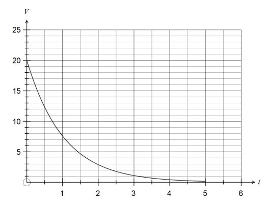
(d) How long, to the nearest millisecond, does it take for the voltage across the capacitor to halve? (2 marks)
